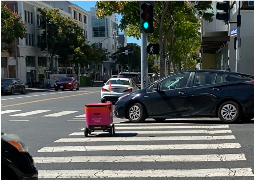
Figure 1: This PMR entered the crosswalk before the right-turn-on-red car entered to block its path. While ISO 4448 stipulates that a PMR shall travel within a marked crosswalk (when it is so marked), and also stipulates that a PMR not reverse or U-turn during a road-crossing maneuver (note in the bottom left corner that another vehicle is turning right behind the PMR). In this circumstance, the PMR subsequently turned out into the roadway to cross in front of the vehicle, breaking the first rule, which, in the circumstance, was the least hazardous rule to ignore, and coincidentally furthered the PMR’s navigational goal of crossing the street. All of this may seem obvious to a teleoperator accustomed to crossing such streets. However, ISO 4448 is intended to set rules, priorities and procedures that will be included in the decision software for these machines.
