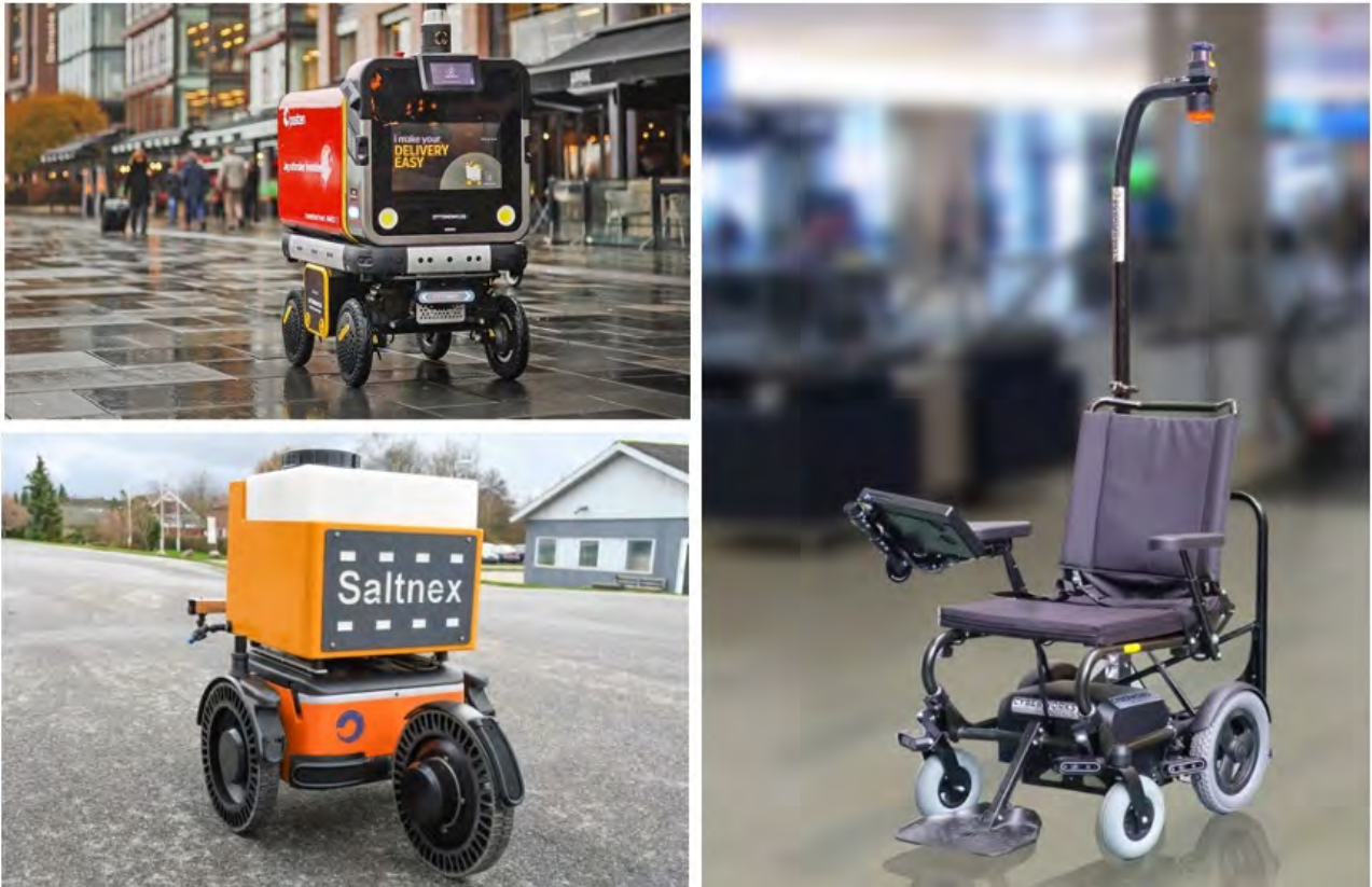
Figure 2: Example form factors of PMRs; Ottobot delivery robot (Ottonomy.io), Saltnex (Capra Robotics), Wheelchair robot (Cyberworks Robotics)
